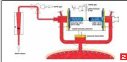
Pressure and temperature are reached in all places of the sterile space (saturated-steam curve 133°C at 2 bar). The steam throughput rate falls to the needed amount in order to maintain the pressure and to compensate the temperature loss by radiation. **Process pressure: 2015 mbar.**
