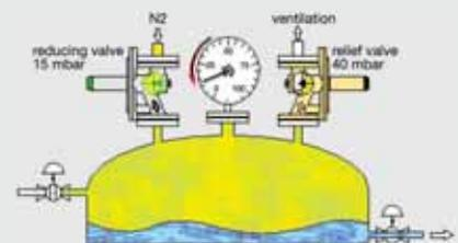
If the reactor cools down or gets emptied, the pressure drops. In case the process pressure falls below the 15 mbar preset on the reducing valve, the reducing valve blows in nitrogen until the pressure reaches 15 mbar again.
