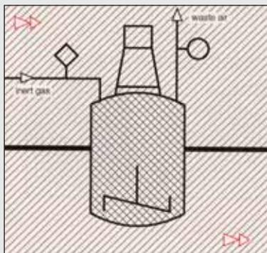
**According to SUVA, change between ZONE 0 and ZONE 1 is possible in apparatus construction under conditions of controlled inertisation.**
