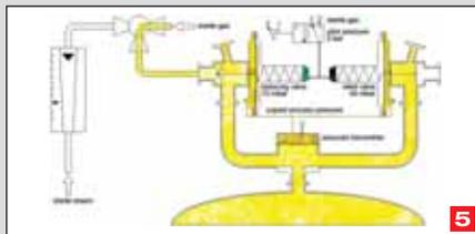
The control system changes over from sterile steam to sterile gas, and the regulators change over to the ventilation mode and maintain sterility of sterile space during the process. **Process pressure: 15 – 40 mbar.**
