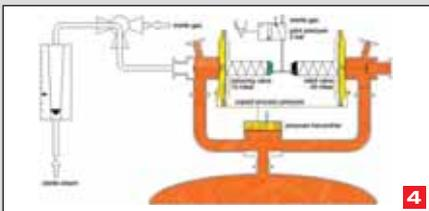
After expiration of holding time, pilot pressure (2 bar) and sterile steam are switched off. The steam pressure is relieved through the relief valve and the production process may start now. **Process pressure: 40 mbar.**
