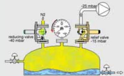
If the reactor cools down or gets emptied, the vacuum pressure rises. If the value of -40 mbar preset on the vacuum-pressure reducing valve is exceeded (e.g. to -43 mbar), the vacuum-pressure reducing valve blows in nitrogen until the process pressure reaches -40 mbar again.
