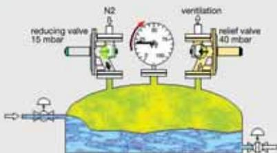
The inertised reactor is filled with the product. The internal pressure rises as a function of the filling level.
