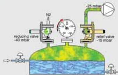
If filling level or temperature level falls below -15 mbar so that the vacuum pressure inside the reactor falls (e.g. to -12 mbar), the vacuum-pressure relief valve evacuates the gas again into the waste air system so that -15 mbar are reached again.
