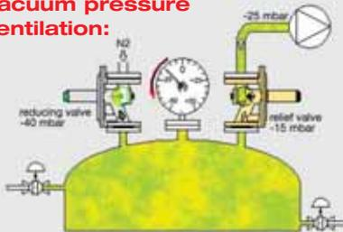
The ventilator evacuates the reactor space through the opened vacuum-pressure relief valve. Once the preset value of -15 mbar is reached, the vacuum-pressure relief valve closes again.
