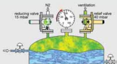
If filling level or temperature level rises so that the reactor pressure exceeds 40 mbar, the relief valve responds and discharges gas into the waste air system.
