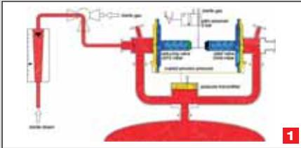
The sterile space is flooded with sterile steam through the opened differential-pressure reducing valve. Both regulators are activated with a pilot pressure of 2 bar. The reducing valve is set to 15 mbar and the relief valve is set to 40 mbar.
