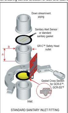
The GCR-SM™ and GCR-SMS™ have a symmetric gasket configuration on both sides of the disk and fit between standard Tri-Clamp® (or equivalent) ferrules.
